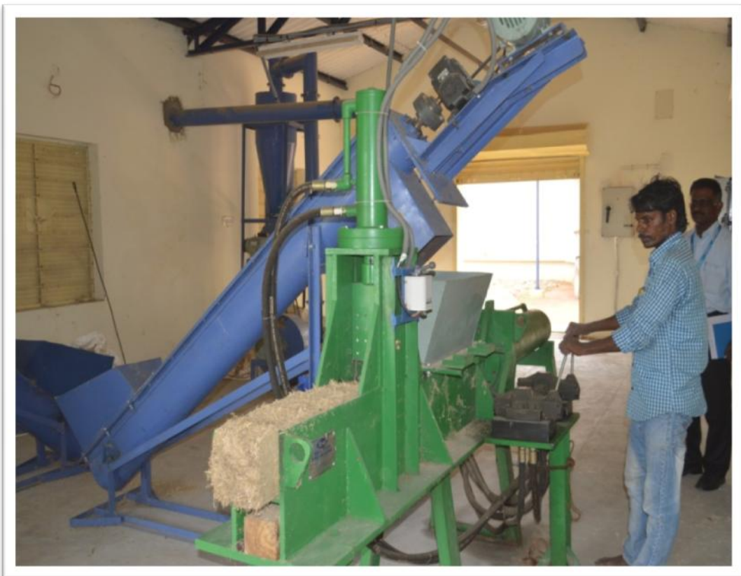
FEED BLOCK MAKING UNIT
